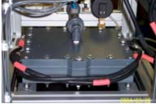
Figure 3. The capacitor cell
